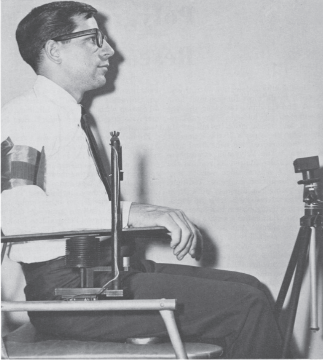
Figure 9. Photograph of a Doppler Non-contact Sensor for Recording Breathing Activity, Reid & Associates, 1960's
